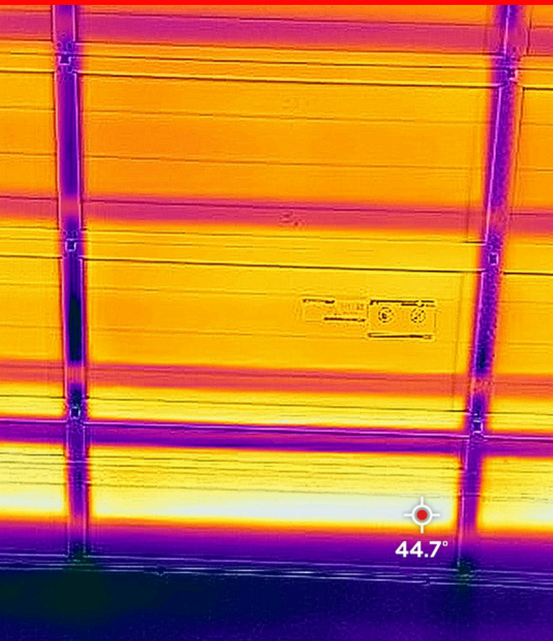
Before: 44.7°C surface temperature Captured at 28°C ambient temperature, Sunshine Coast QLD
